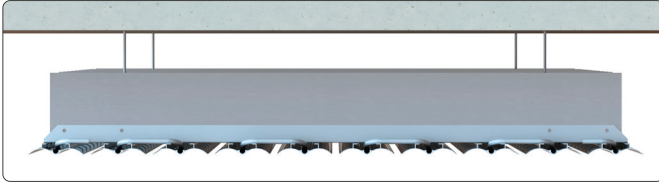
Front view; Baffles placed across the fins
